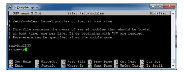
Save the file and reboot the Pi with **sudo reboot** and look at the console output (or run **dmesg** in the console window after logging in) you will see the modules install. Look in particular for the STMPE610 detection and the ILI9340 screen frequency as highlighted here
