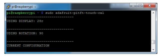
By default the script will attempt to read the screen orientation by examining the PiTFT module configuration with modprobe. If the script can read the orientation it will print out the current orientation, the current touchscreen calibration values, and the new touchscreen calibration values baesd on the current orientation. Before updating the calibration the script will ask you to confirm that you'd like to make the change. Press **y** and enter to confirm.
