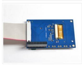
You can attach a 26-pin IDC cable just make sure the pin 1 indicator is on the right as indicated in this photo - there's also a #1 marking on the PCB!
