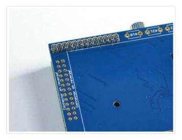
Before attaching the display, check that all the pins are soldered nicely and there's no bridging, cold
