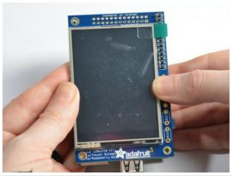
Once you have the screen so it is definitely not touching the header, you can gently press on the sides to secure the tape.
