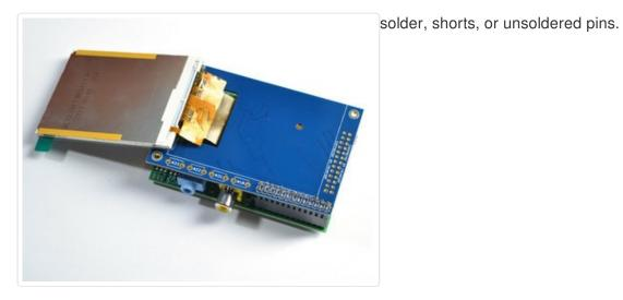
Now we can attach the screen. Remove the two thin tape cover strips.
