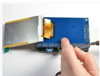
Heat up your soldering iron, and grab some solder. Start by tack-soldering one of the corners while pressing on the plate to make it sit flat. Once you have one or two pins done you can continue to solder each of the pins.
