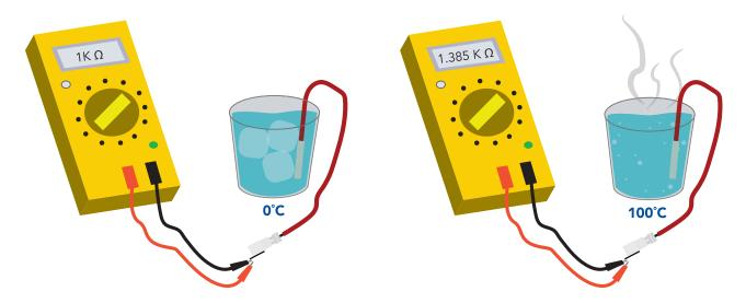
To convert the resistance of the probe to temperature the use the following simplified equation:
