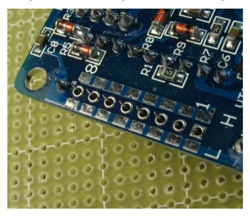
And setup the corresponding pins on PT2272:
