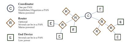
In ZigBee networks, the coordinator must select a PAN ID (64-bit and 16-bit) and channel to start a network. After that, it behaves essentially like a router. The coordinator and routers can allow other devices to join the network and can route data.
