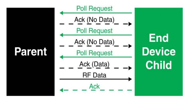
If the end device receives the acknowledgment and finds that the parent has no data for it, the end device can return to idle mode or sleep. Otherwise, it will remain awake to receive the data. This polling mechanism allows the end device to enter idle mode and turn its receiver off when RF data is not expected in order to reduce current consumption and conserve battery life.
