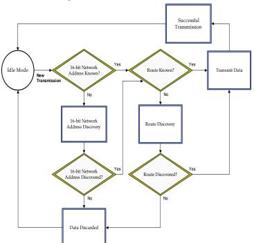
When data is transmitted from one node to another, a network-level acknowledgement is transmitted back across the established route to the source node. This acknowledgement packet indicates to the source node that the data packet was received by the destination node. If a network acknowledgement is not received, the source node will re-transmit the data.
