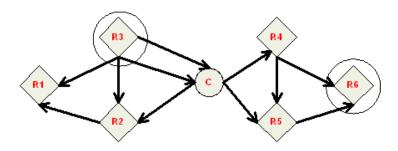
When the destination node receives a route request, it compares the 'path cost' field against previously received route request commands. If the path cost stored in the route request is better than any previously received, the destination node will transmit a route reply packet to the node that originated the route request. Intermediate nodes receive and forward the route reply packet to the source node (the node that originated route request).
