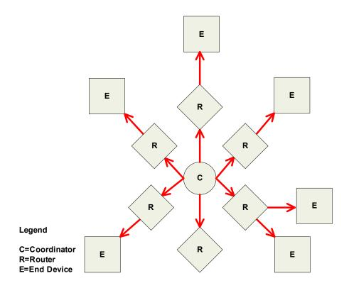
Each node that transmits the broadcast will also create an entry in a local broadcast transmission table. This entry is used to keep track of each received broadcast packet to ensure the packets are not endlessly transmitted. Each entry persists for 8 seconds. The broadcast transmission table holds 8 entries.
