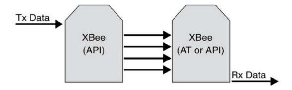
The API transmit frame can include up to 255 bytes of data, which will be broken up into multiple transmissions and reassembled on the receiving side. If one or more of the fragmented messages are not received by the receiving device, the receiver will drop the entire message, and the sender will indicate a transmission failure in the Tx Status API frame. ZB firmware can only support one fragmented packet at a time at the receive node, due to memory constraints.
