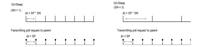
Setting SN > 1 allows the XBee to silently poll for data without asserting On /Sleep. If RF data is received when polling, On/Sleep will immediately assert.
