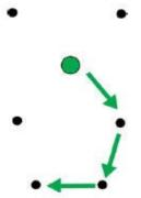
A remote device sends an RF data packet to the data collector. (This is prefaced by a route record transmission to the data collector.)
