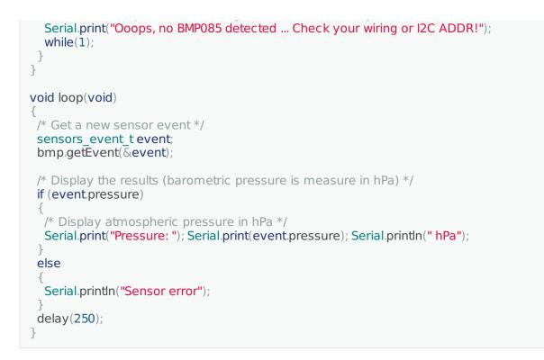
Then open up the serial monitor at 9600 baud. The sketch will continuously print out the pressure in **hPa** (hectoPascals). You can test that the sensor is measuring variations in pressure by placing your fingertip over the open port hole in the top of the sensor. The pressure will increase as you can see here:
