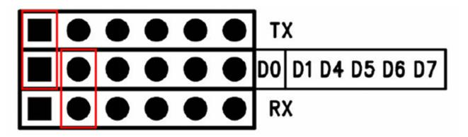
Then the serial data lines from the bluetooth module will be sending and receiving with the TX/RX uart interface on the arduino chip. This is the mode you normally use to do bluetooth communications with the arduino from some external bluetooth device such as a smartphone that talks over a serial bluetooth profile (RFCOMM).
