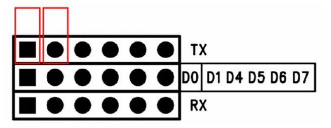
That just uses the pins as a place to store the jumpers, but not have them connecting anything, and it makes it safe to use the USB serial interface for comunicating with the arduino.
